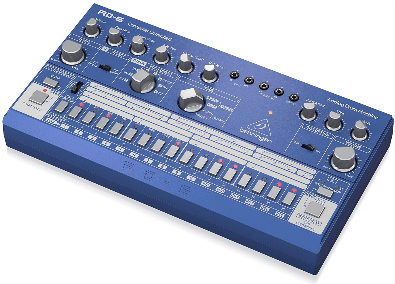
Figure 2: Behringer RD-6 front panel. This image shows the tempo knob, accent control, individual drum voice controls, mode selector, step buttons, and distortion section.
