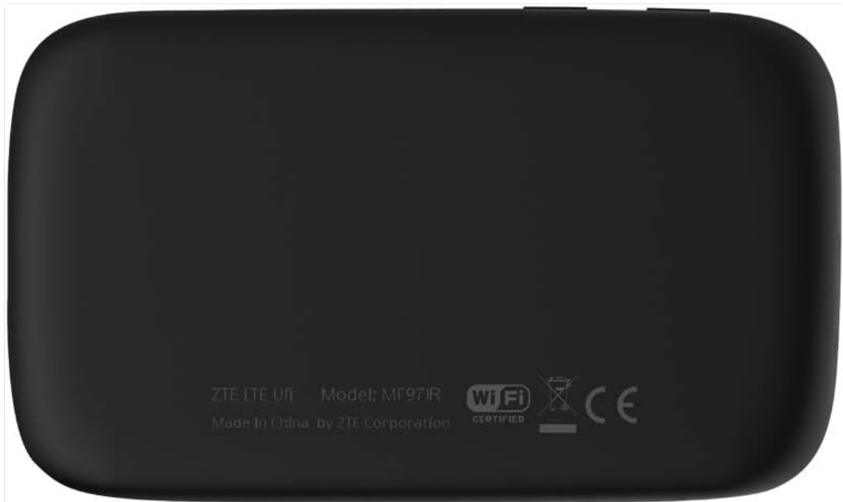
Figure 3.2: Rear view of the ZTE MF971R hotspot, displaying model information and certifications.
