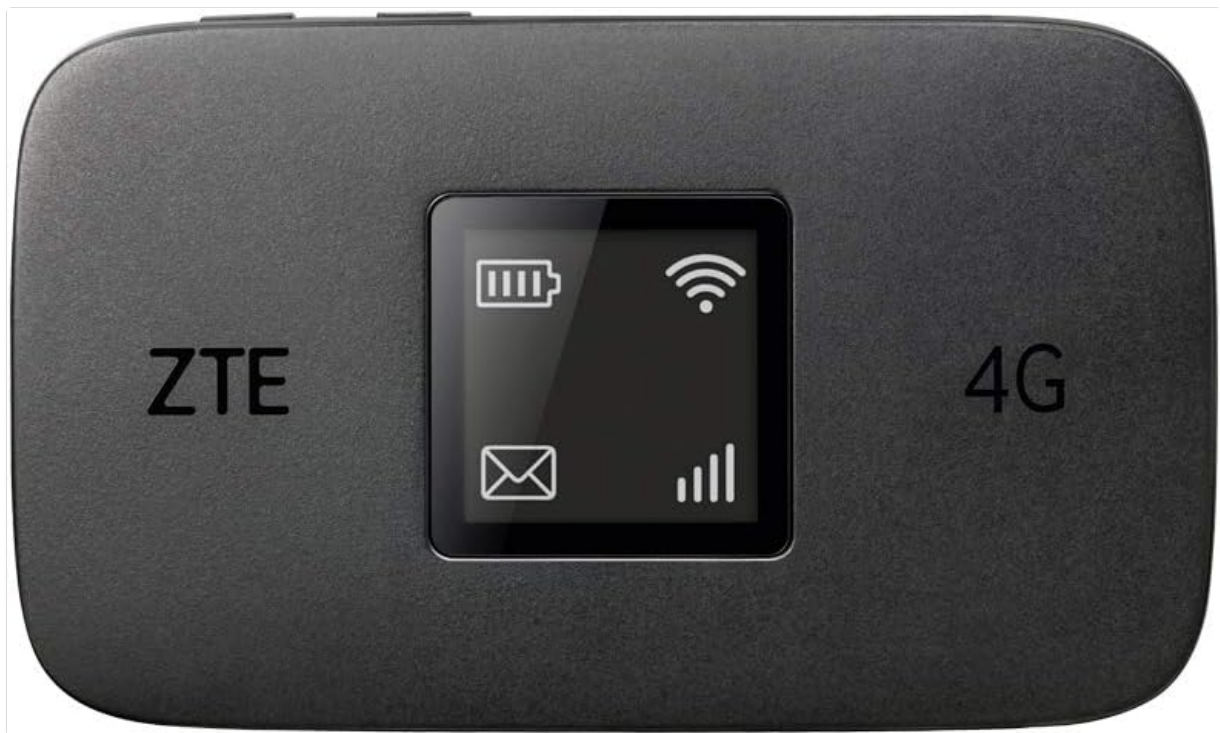
Figure 3.1: Front view of the ZTE MF971R hotspot, showing the screen with battery, Wi-Fi, and signal indicators.
