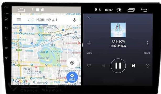
Figure 4: The 10.1-inch display showcasing multi-window functionality and the adjustable viewing angle mechanism.
