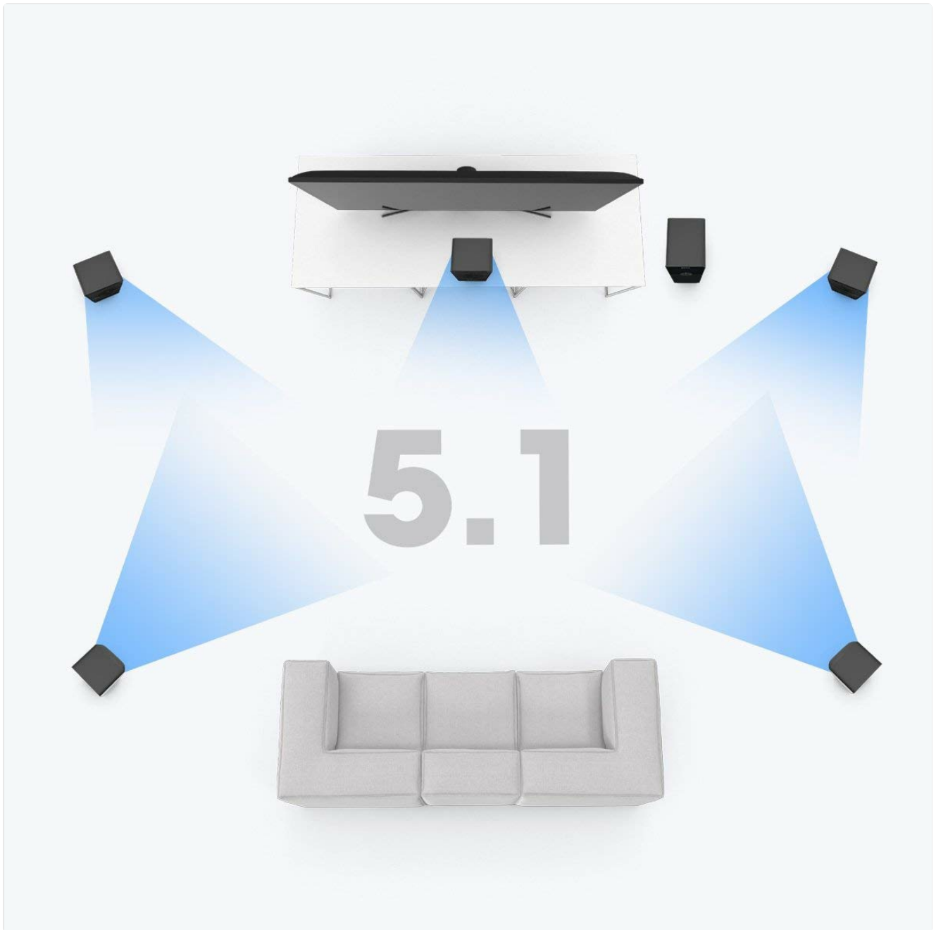
Image: A diagram showing the recommended 5.1 speaker setup, with the subwoofer and five satellite speakers strategically placed around a listening area for optimal surround sound.
