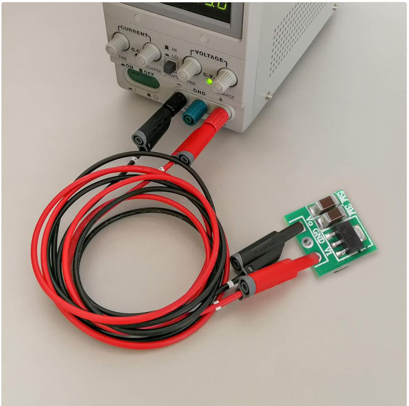
Image 5.1: An example setup showing the DC-DC Step-Up Power Module connected to a power supply for input and a multimeter for output voltage measurement, illustrating typical wiring.
