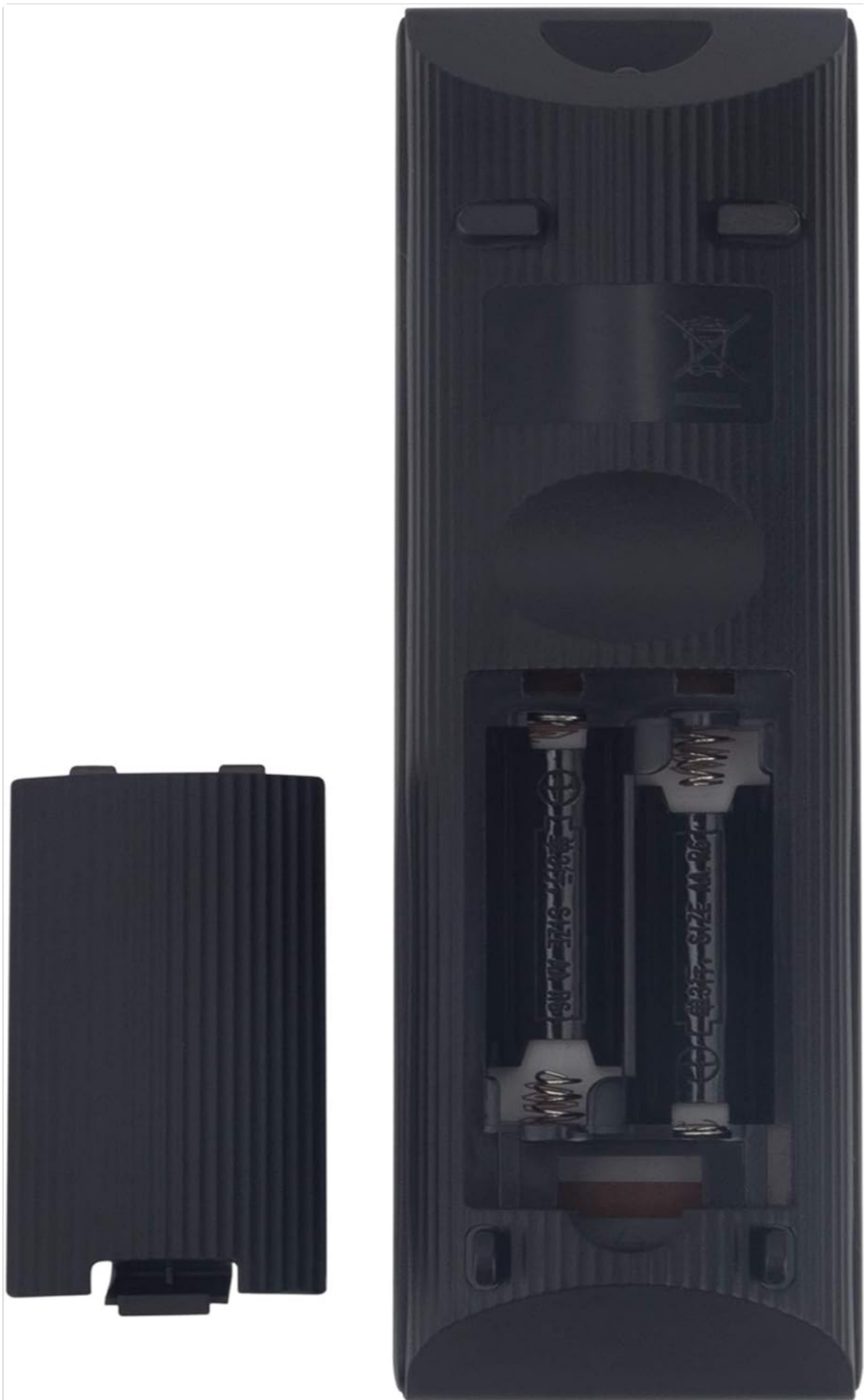
Image 2.1: Back view of the remote control with the battery cover removed, illustrating the battery insertion process.
