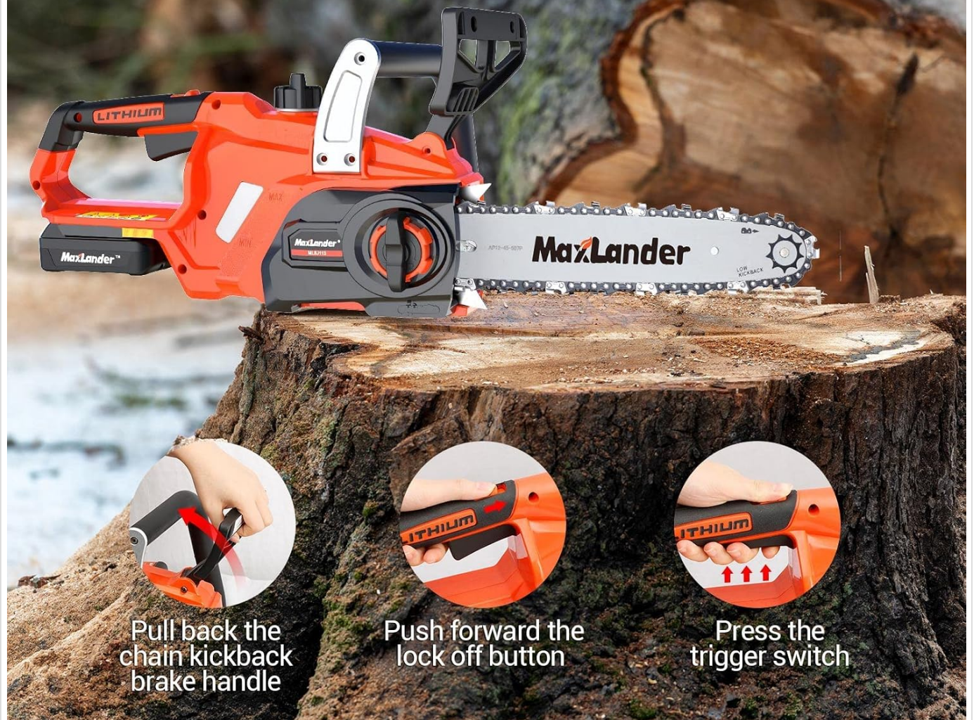
Image 6.1: A visual guide illustrating the three safety steps required to start the chainsaw: pulling back the chain kickback brake handle, pushing forward the lock-off button, and simultaneously pressing the trigger switch.
