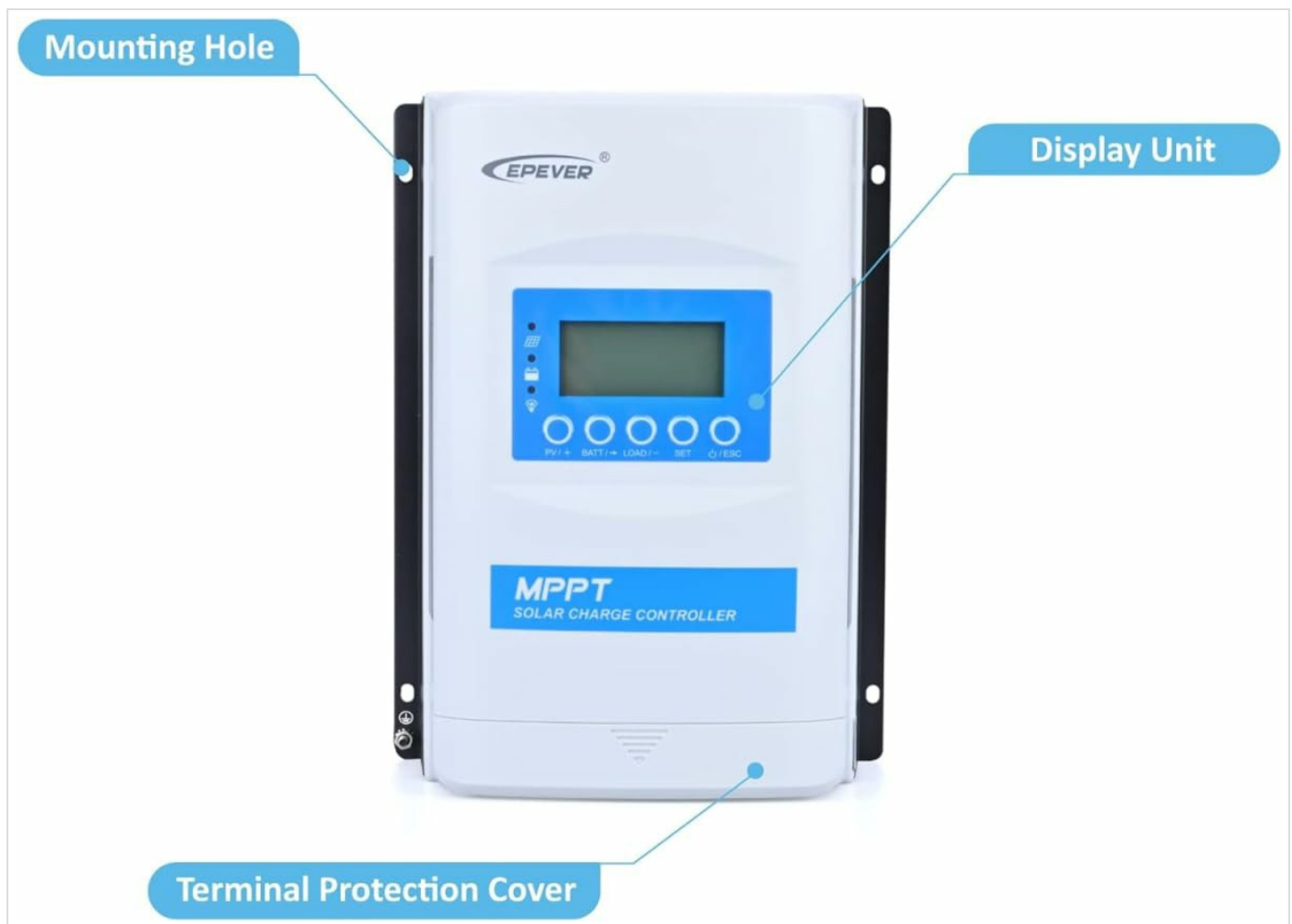
Figure 5.1: Front View with Mounting Hole and Display Unit
