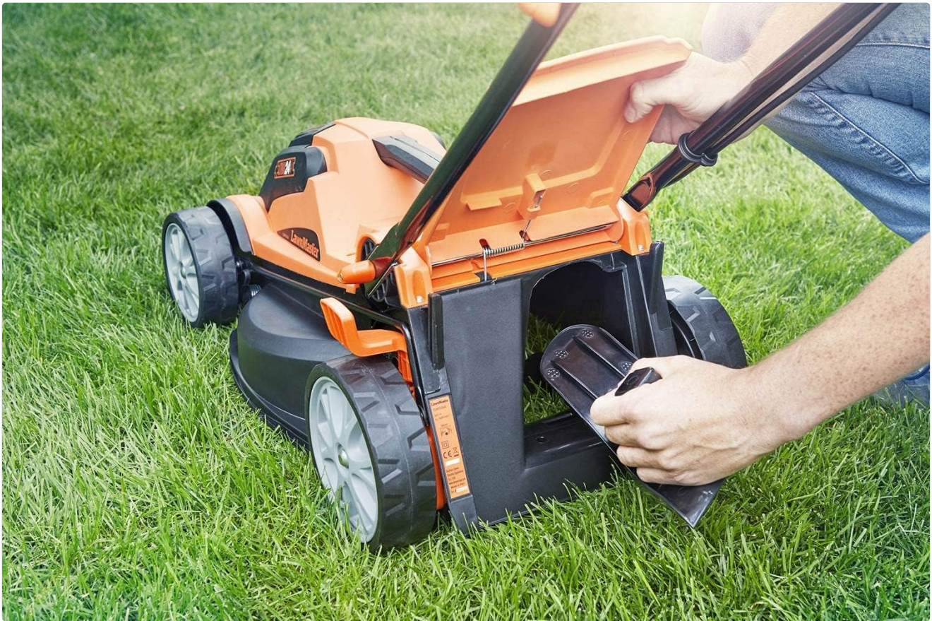
Figure 5.2: Inserting the mulching plug for nutrient return to the lawn.
