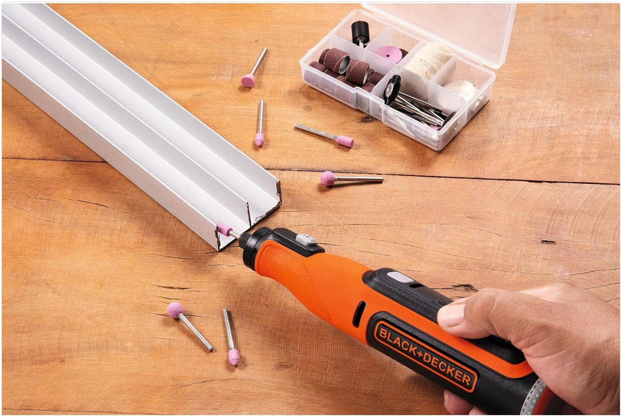
Image 9: The rotary tool with a grinding stone, precisely shaping the edge of a plastic channel.
