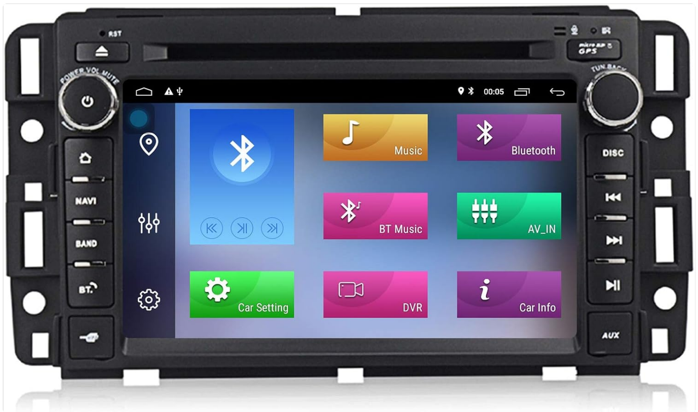
Figure 4.1: The main user interface of the car stereo, displaying icons for Music, Bluetooth, Car Setting, DVR, Car Info, and AV_IN.
