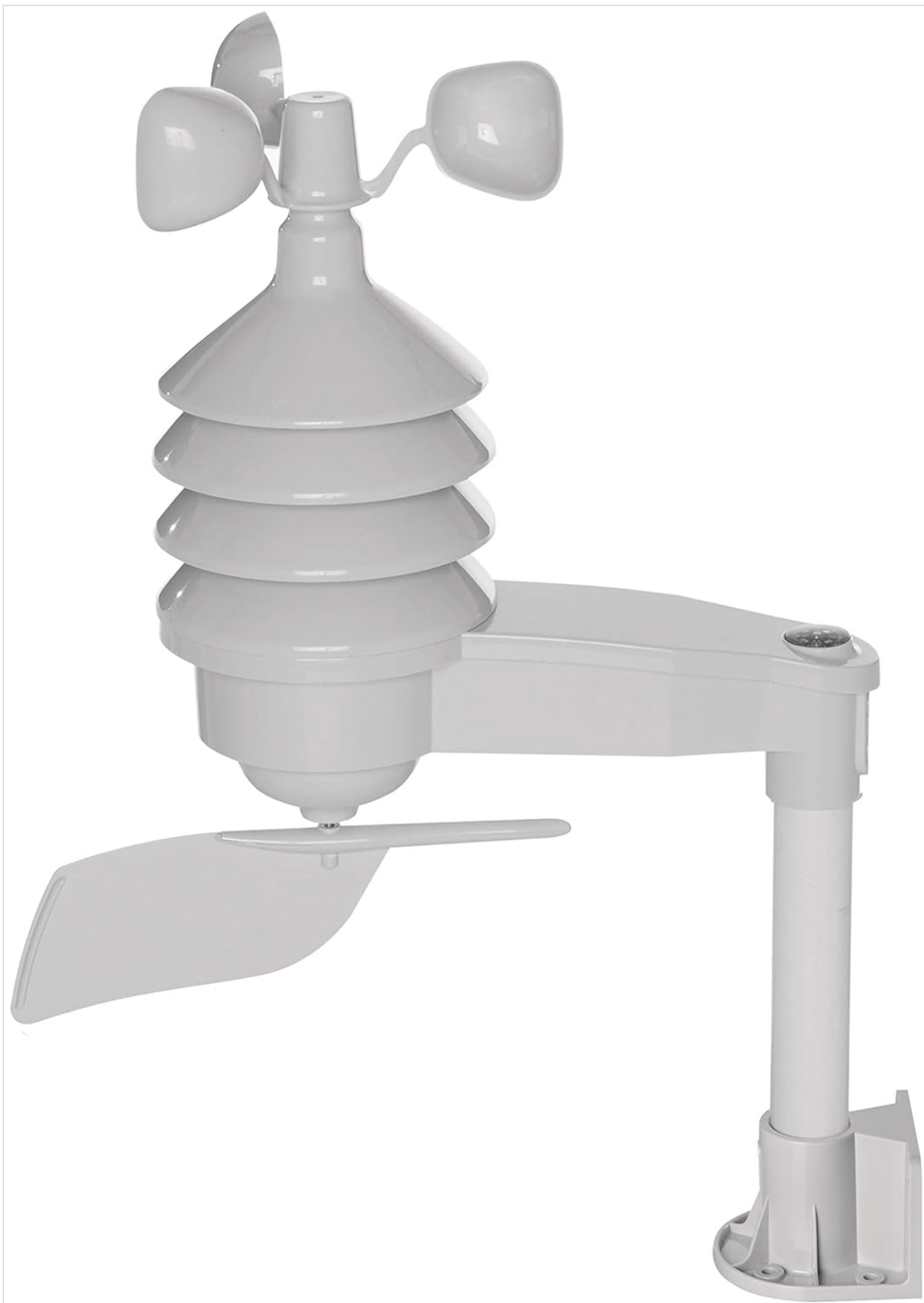
Figure 1: EMOS E06016 Wireless Wind Sensor. This image shows the complete assembly of the wind sensor, including the anemometer cups for wind speed, the wind vane for wind direction, and the radiation shields for temperature and humidity sensing.
