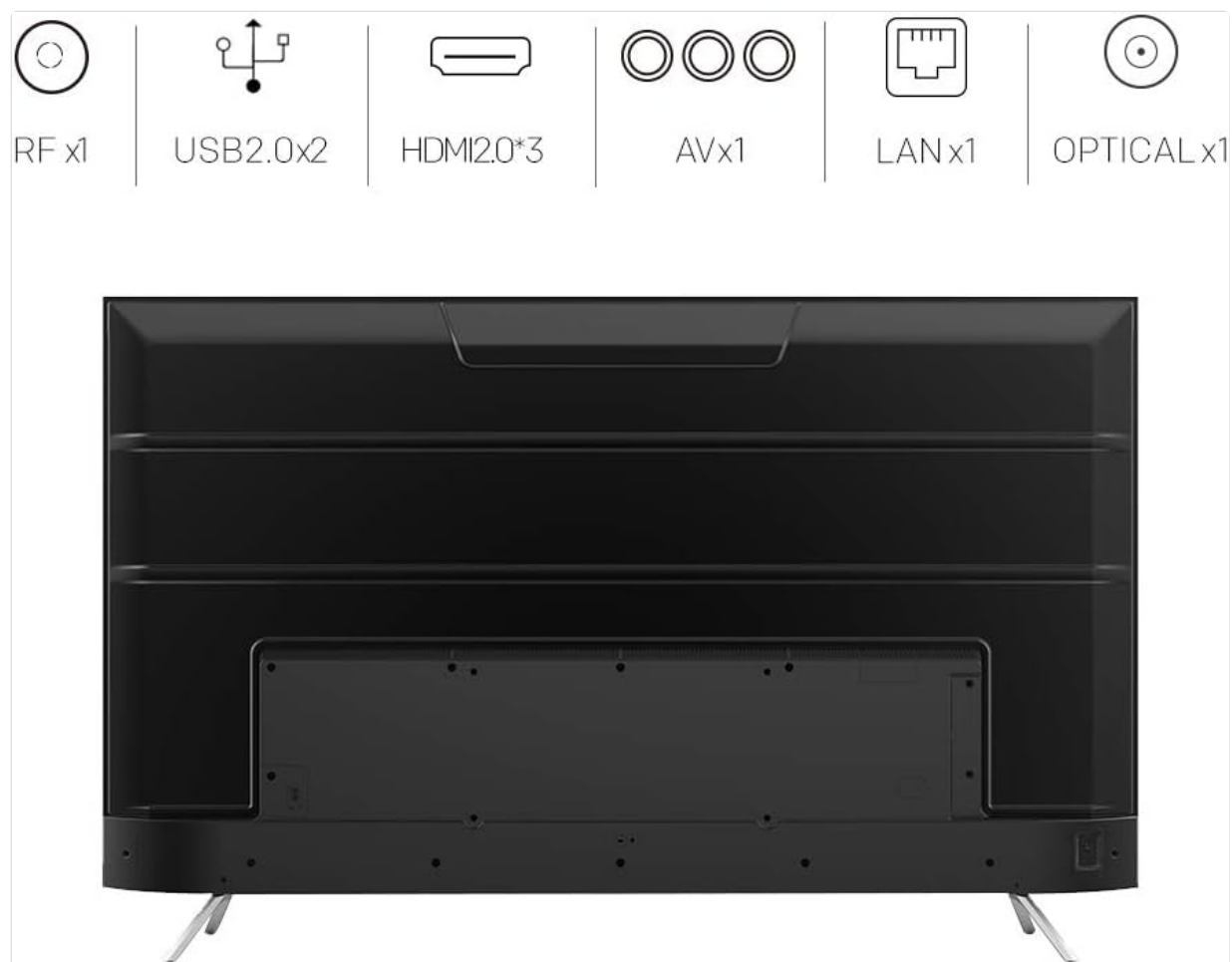
Image: Rear view of the Metz MUC7000 TV, illustrating the location of connectivity ports including RF, USB, HDMI, AV, LAN, and Optical audio out.
