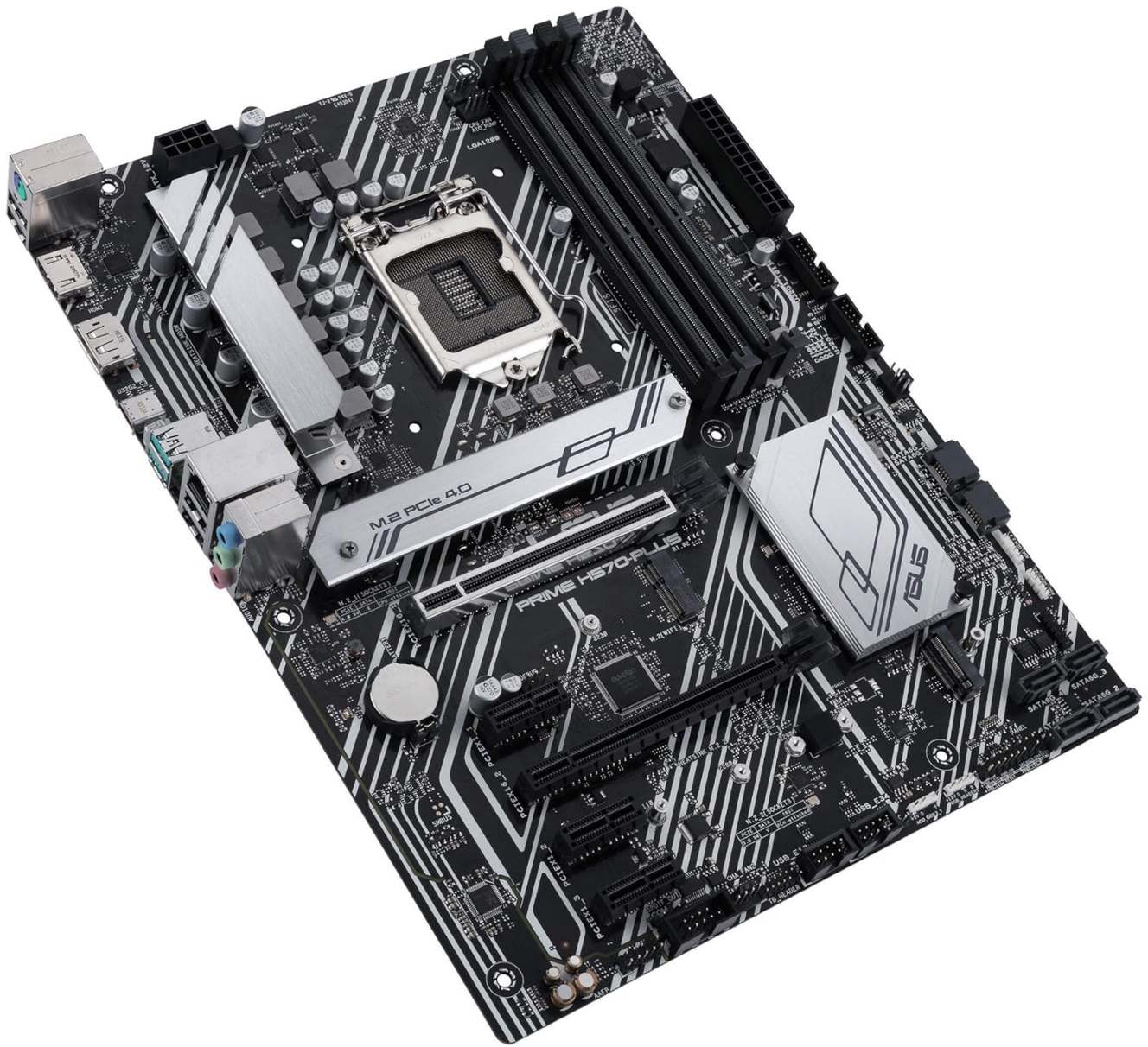
Image 4.2: Top-down angled view, showing PCIe slots and SATA ports.
