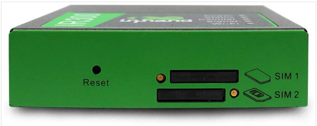
Figure 4.3: Side Panel with SIM Slots. One side of the router features a recessed Reset button and two accessible SIM card slots, labeled SIM 1 and SIM 2 , allowing for dual-SIM redundancy.
