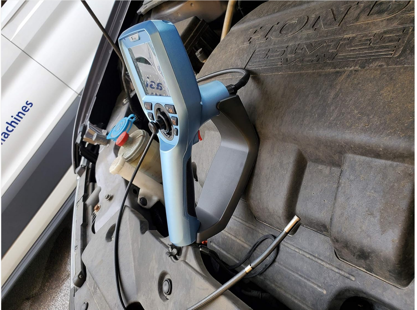
Image 6.1: The Vividia ME-630 videoscope being used for an automotive inspection, demonstrating its practical application.
