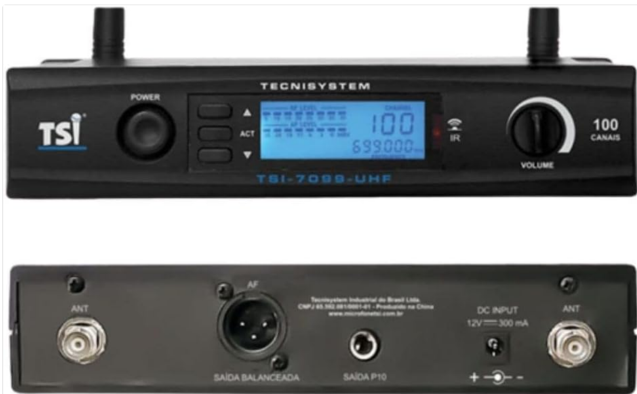
Figure 2.1: Front and rear view of the TSI UD7099 receiver unit, showing controls, display, antennas, and audio outputs.
