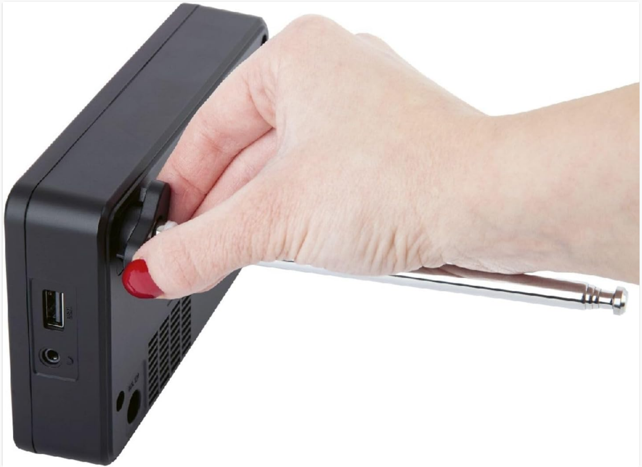
Image: A hand extending the telescopic antenna from the side of the Telestar DIRA M 6i radio, showing the USB port and headphone jack.
