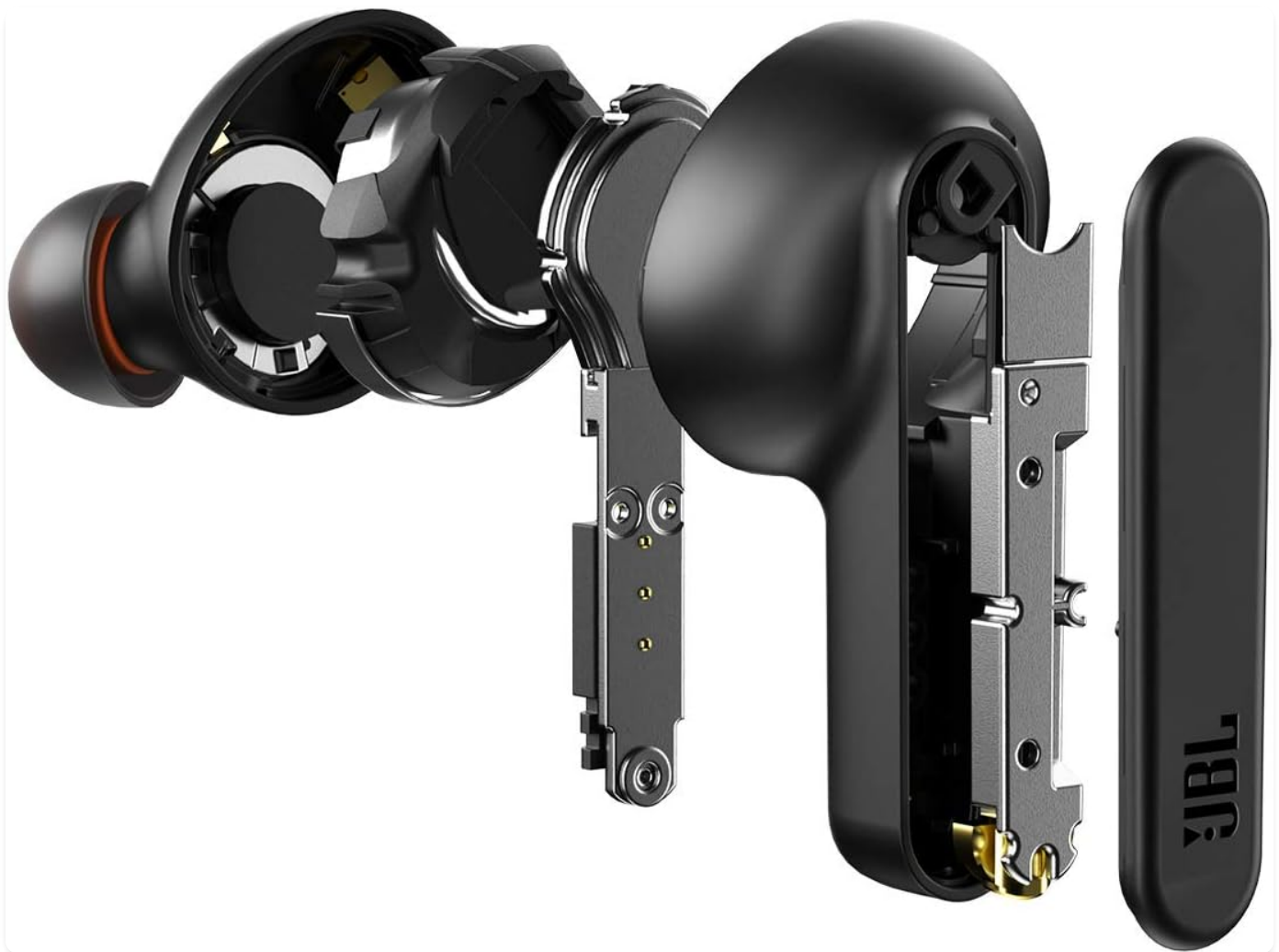
Figure 7.1: Internal components of an earbud.
