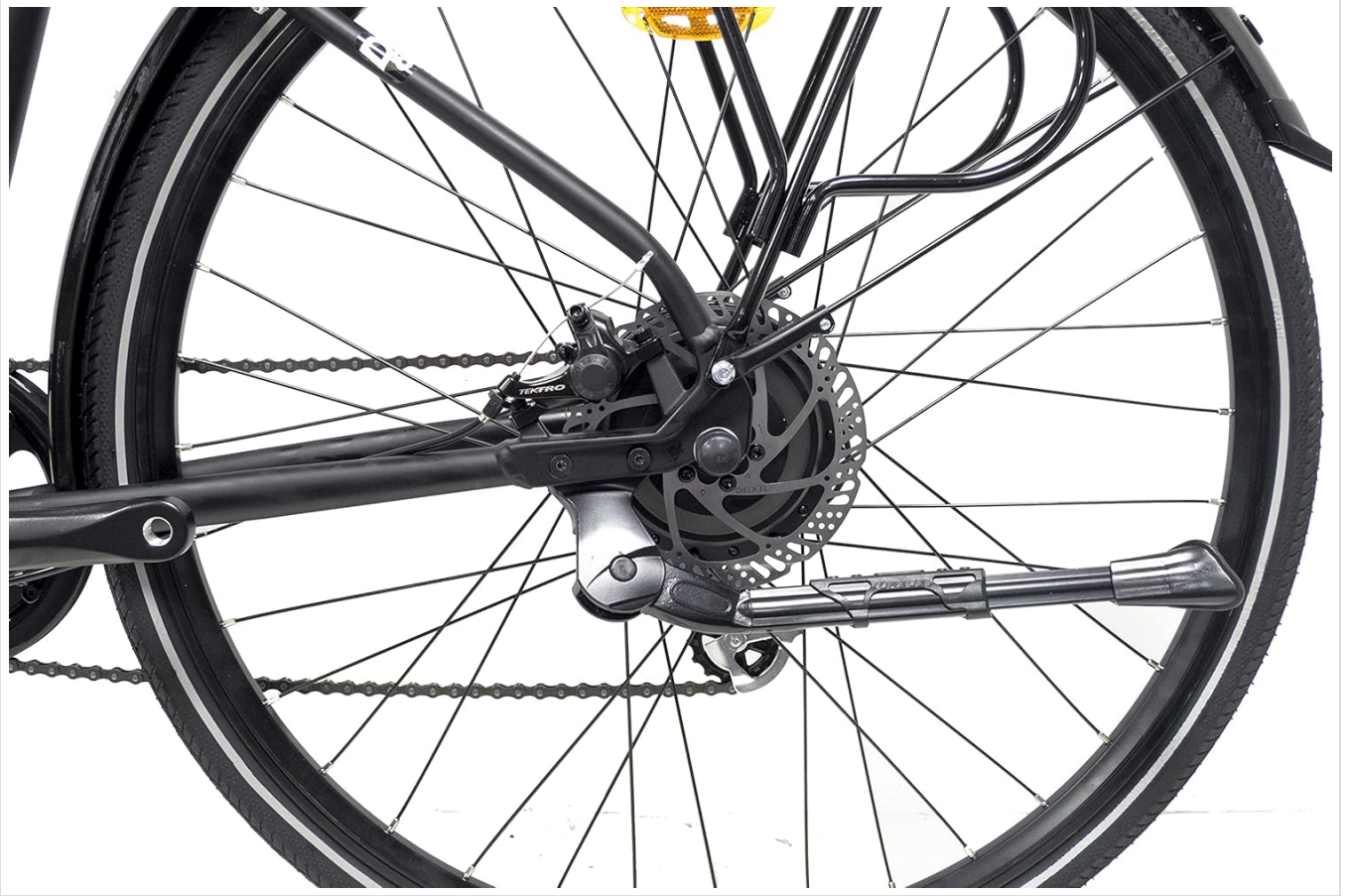
Figure 6: Rear disc brake and motor assembly.
