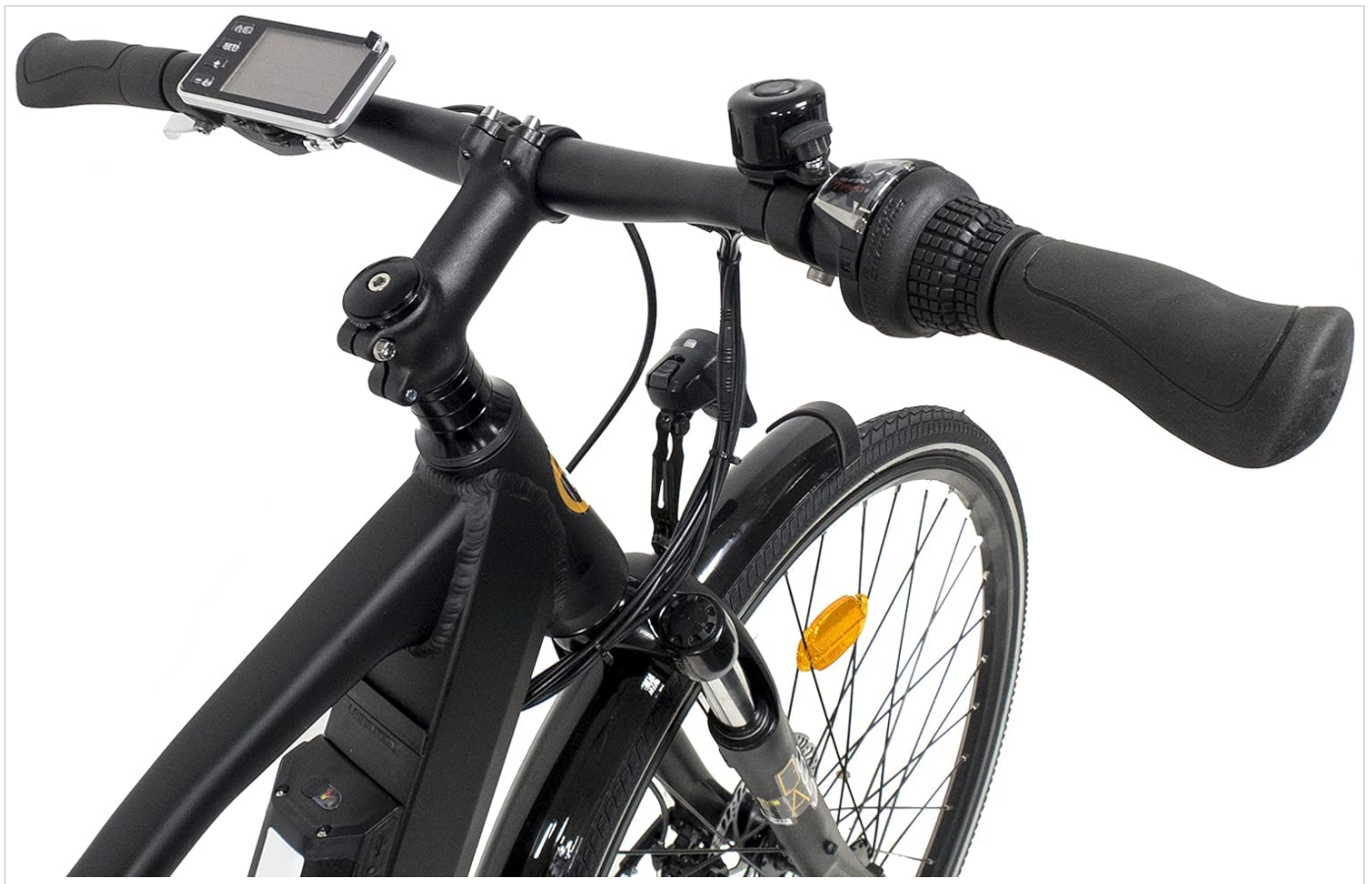
Figure 3: Detailed view of the handlebar, showing the display unit and controls for initial setup.
