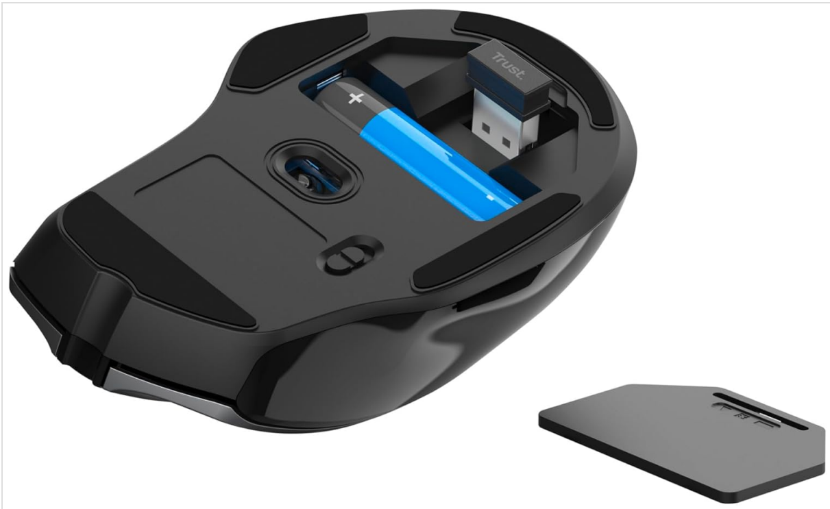
Image 4.2: Bottom view of the Trust Wireless Mouse, illustrating the battery compartment and the storage slot for the USB micro receiver.
