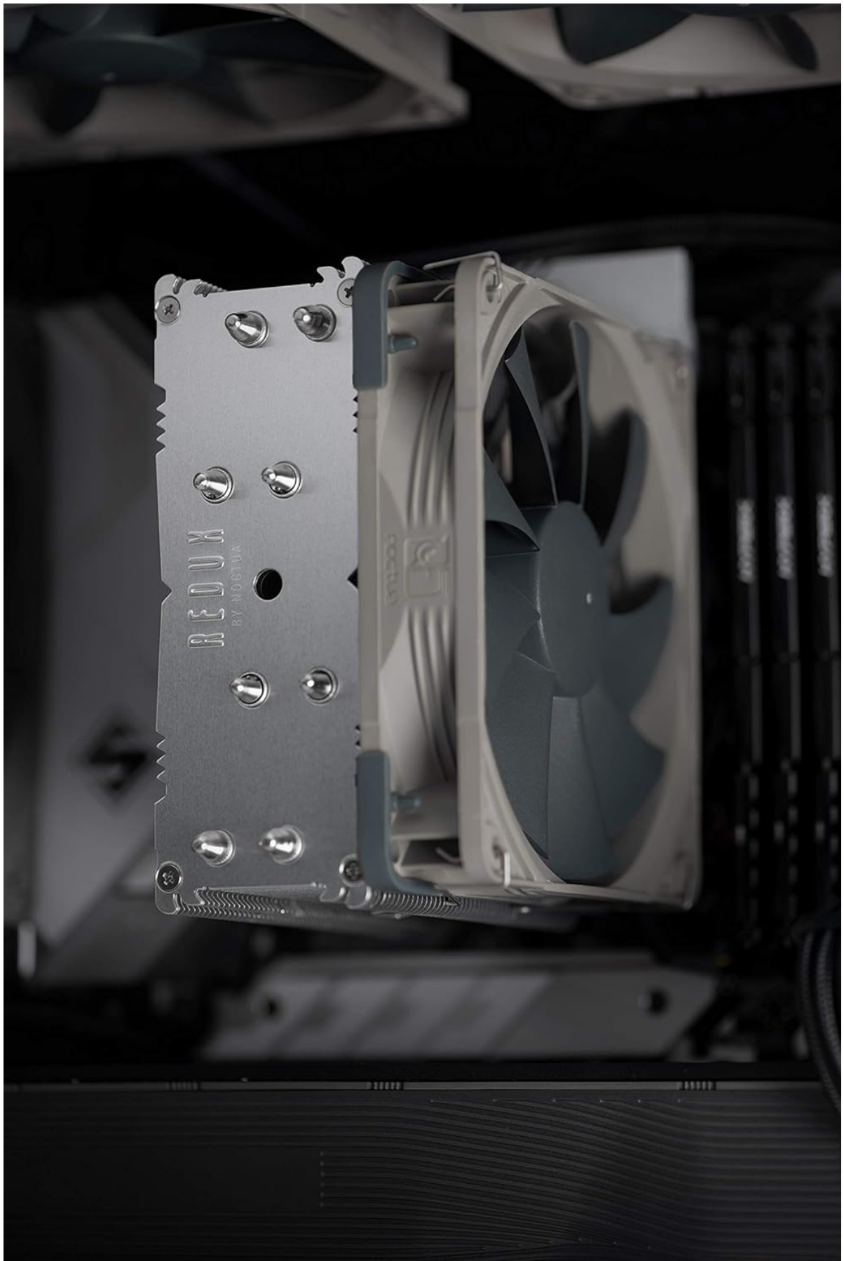
Image: The Noctua NH-U12S Redux CPU cooler installed within a computer case, demonstrating its compact form factor and clearance around memory modules.
