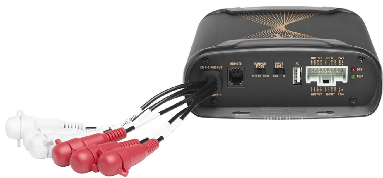
Figure 3: A detailed view of the INFDSP4425's control panel, showing the remote port, turn-on mode switch (REM, DC, AUDIO), input level switch (LOW, HI), PC connection port, and the output/input wiring terminals.
