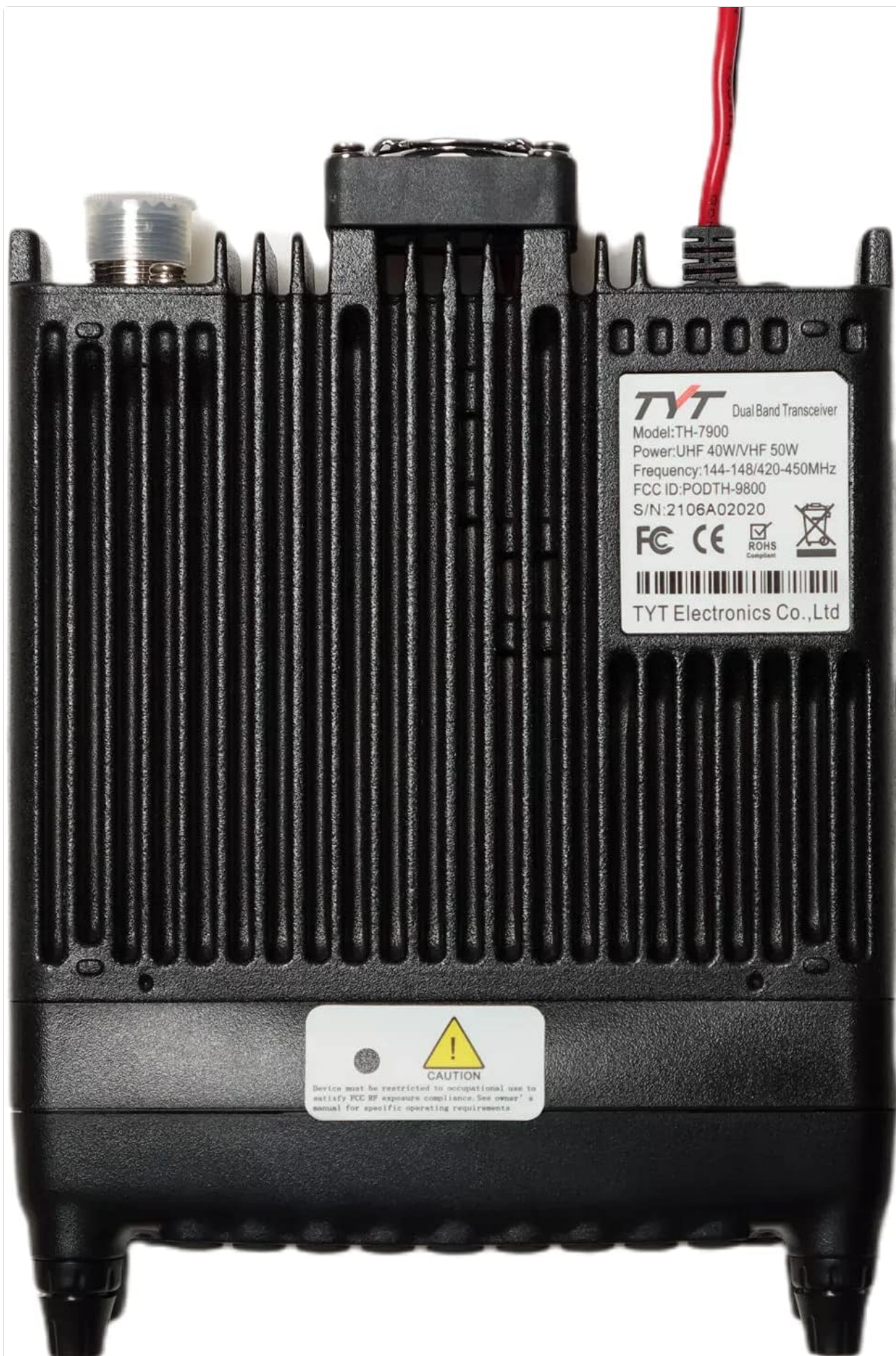
Figure 4.3: Bottom view of the TH-7900, displaying the product label with Model: TH-7900, Power: UHF 40W/VHF 50W, Frequency: 144-148MHz/420-450MHz, FCC ID: PODTH-9800, and S/N: 2106A02020.
