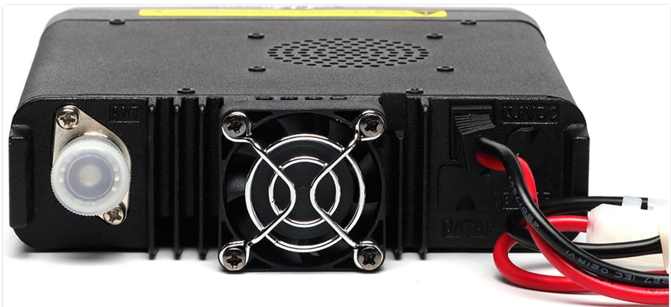
Figure 4.2: Rear view of the TH-7900, highlighting the antenna port, cooling fan, and DC power input.
