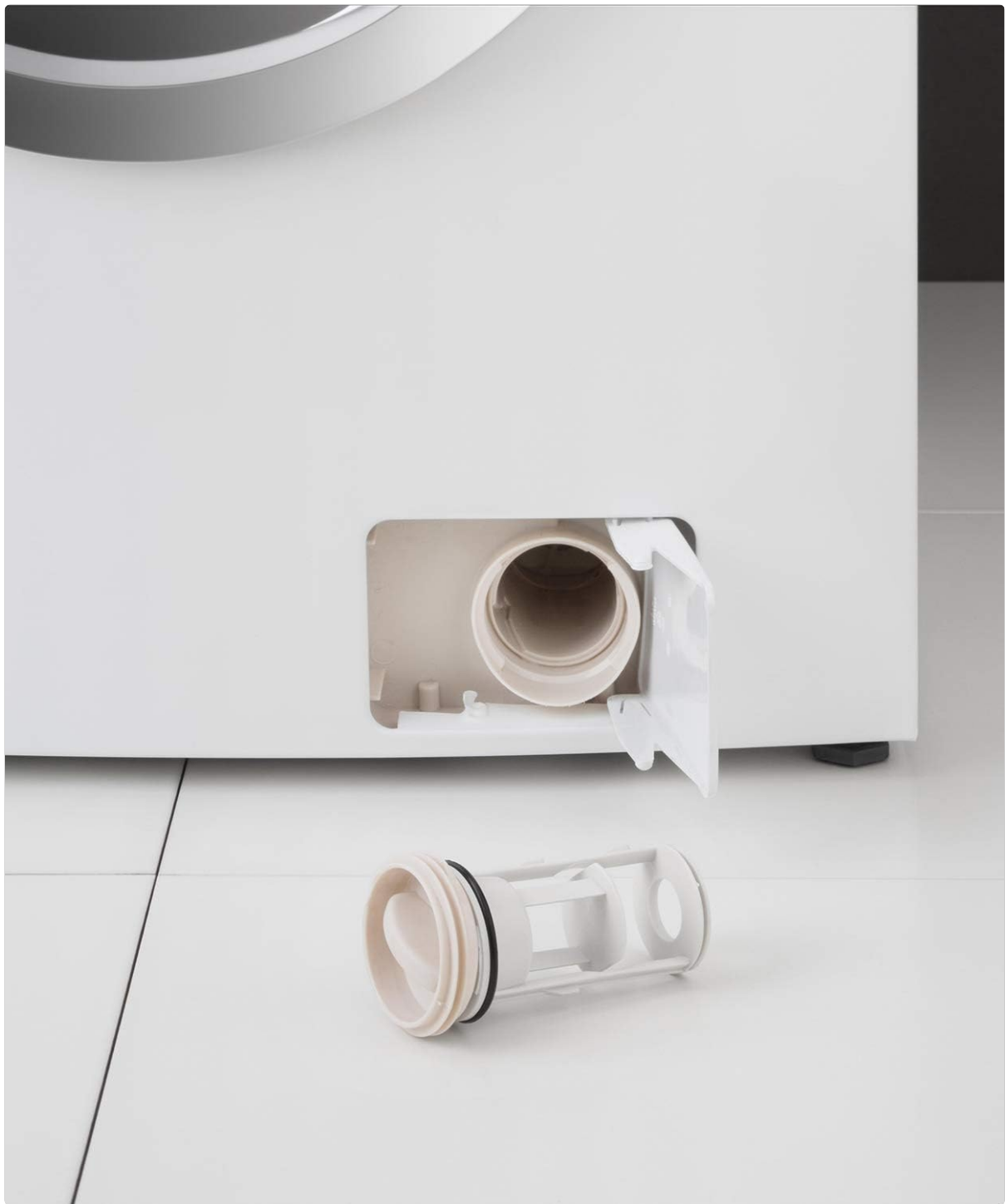
Figure 3.6: The drain pump filter and its access panel located at the bottom front of the washing machine. The filter is designed to collect lint and small objects, preventing them from clogging the pump.
