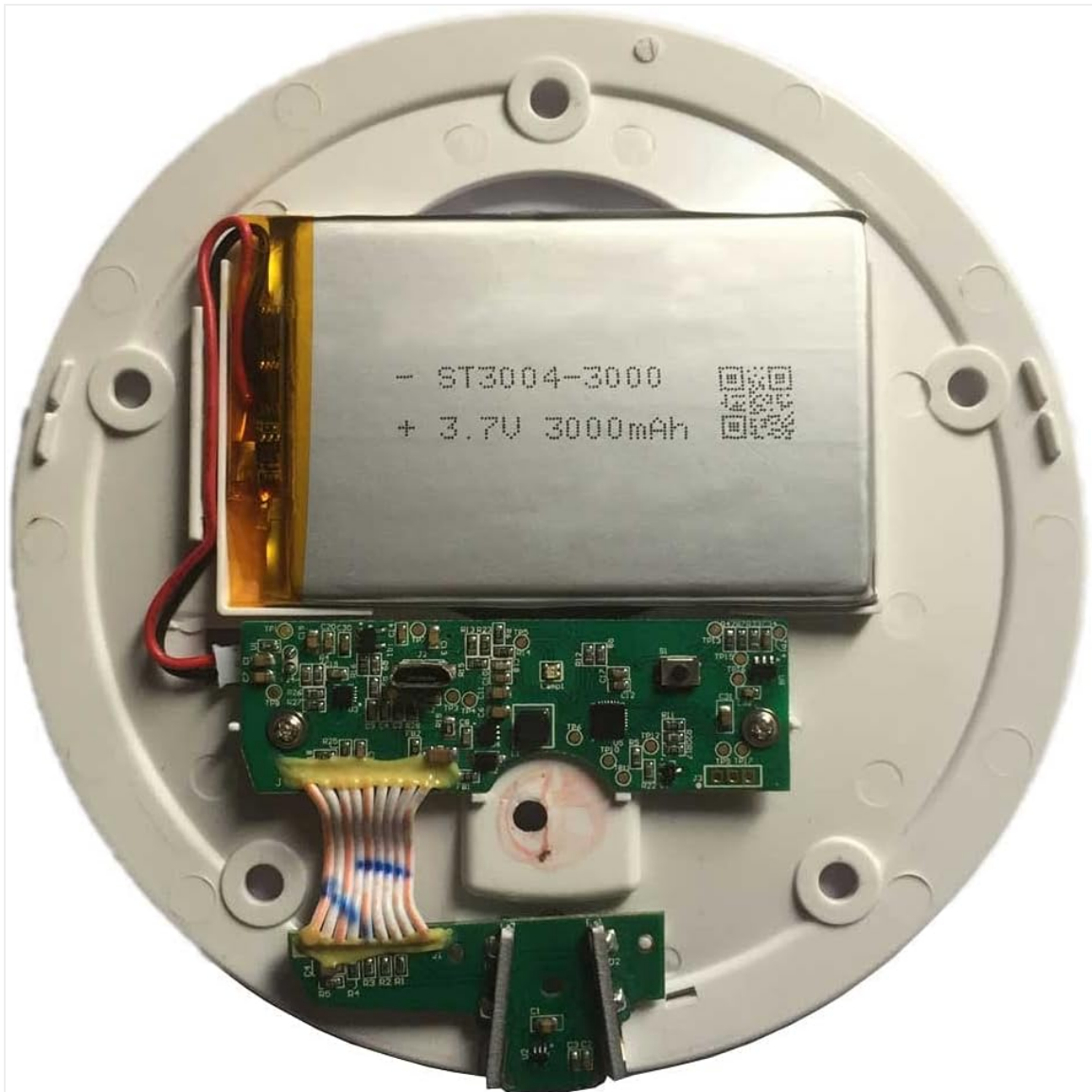
Image: The AOLIKES 3.7V 3000mAh Lithium Polymer Replacement Battery connected to the circuit board within a Simplehuman mirror base.
