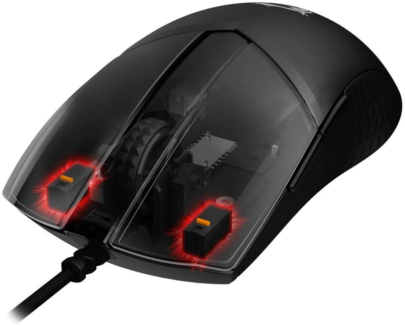
Figure 7: Internal view showing the OMRON switches.
