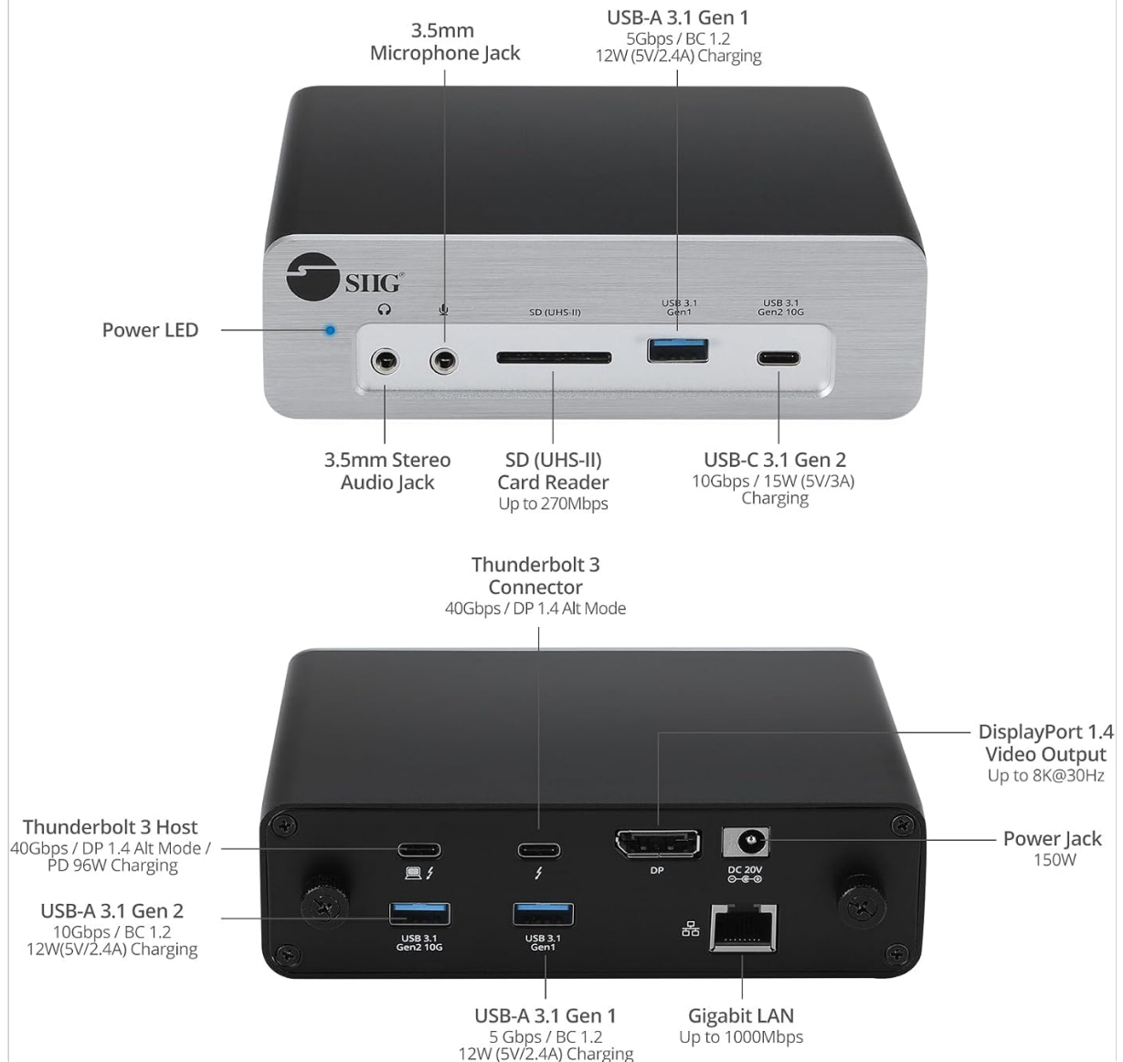
Image: Front and rear panel connections of the SIIG Thunderbolt 3 Dock.
