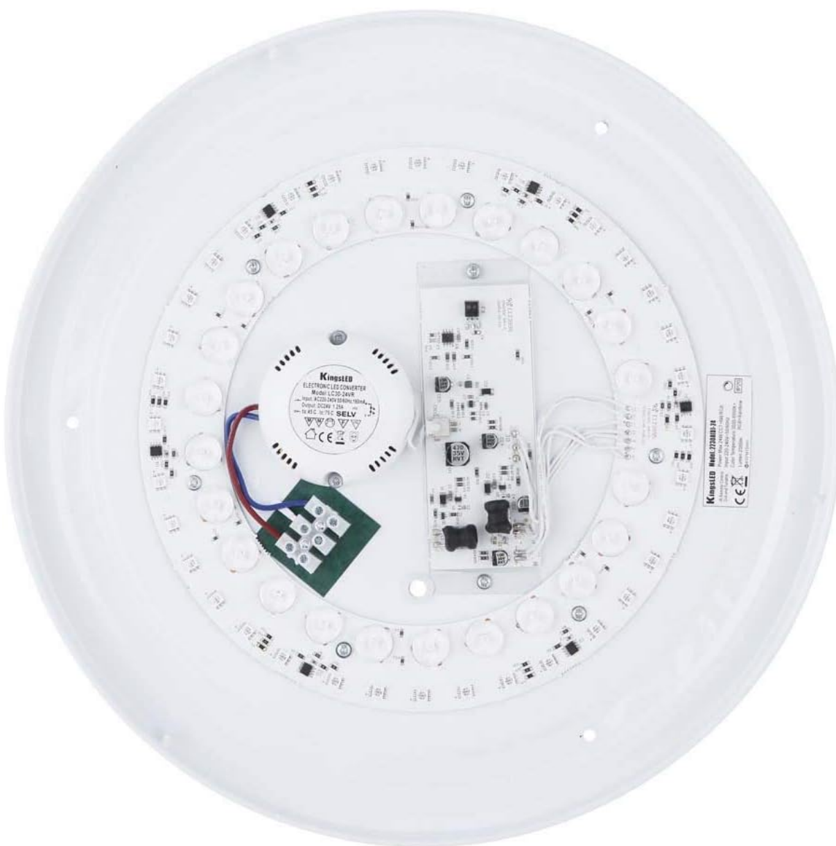
Image 5.1: Internal view of the lamp showing the LED driver and wiring terminals. Ensure connections are made according to local electrical codes.
