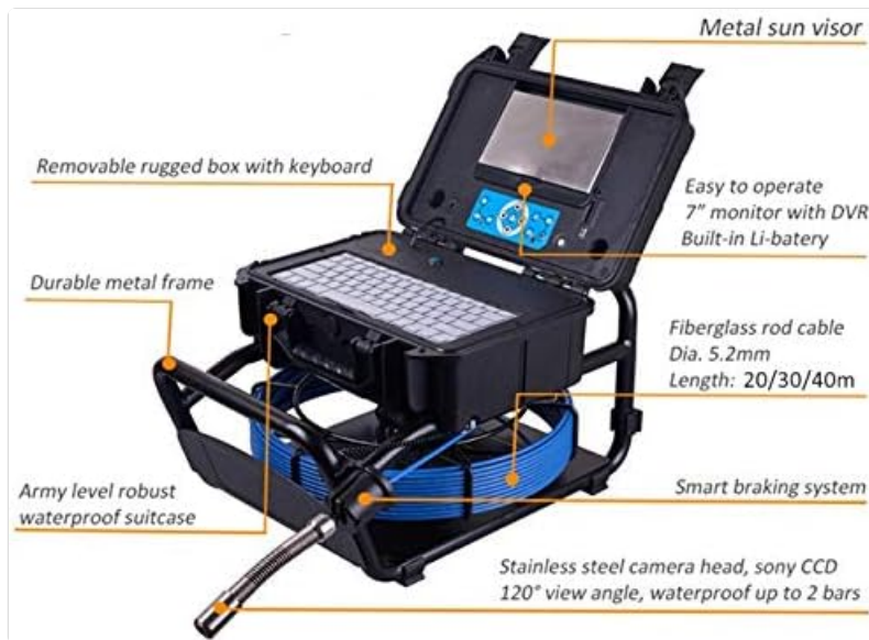
Figure 3: Control box mounted on the cable reel frame.
