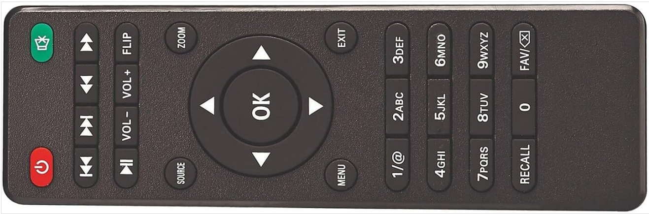
The remote control for the RCA 480P Home Movie Projector, showing button layout for power, navigation, volume, source selection, and other functions.
