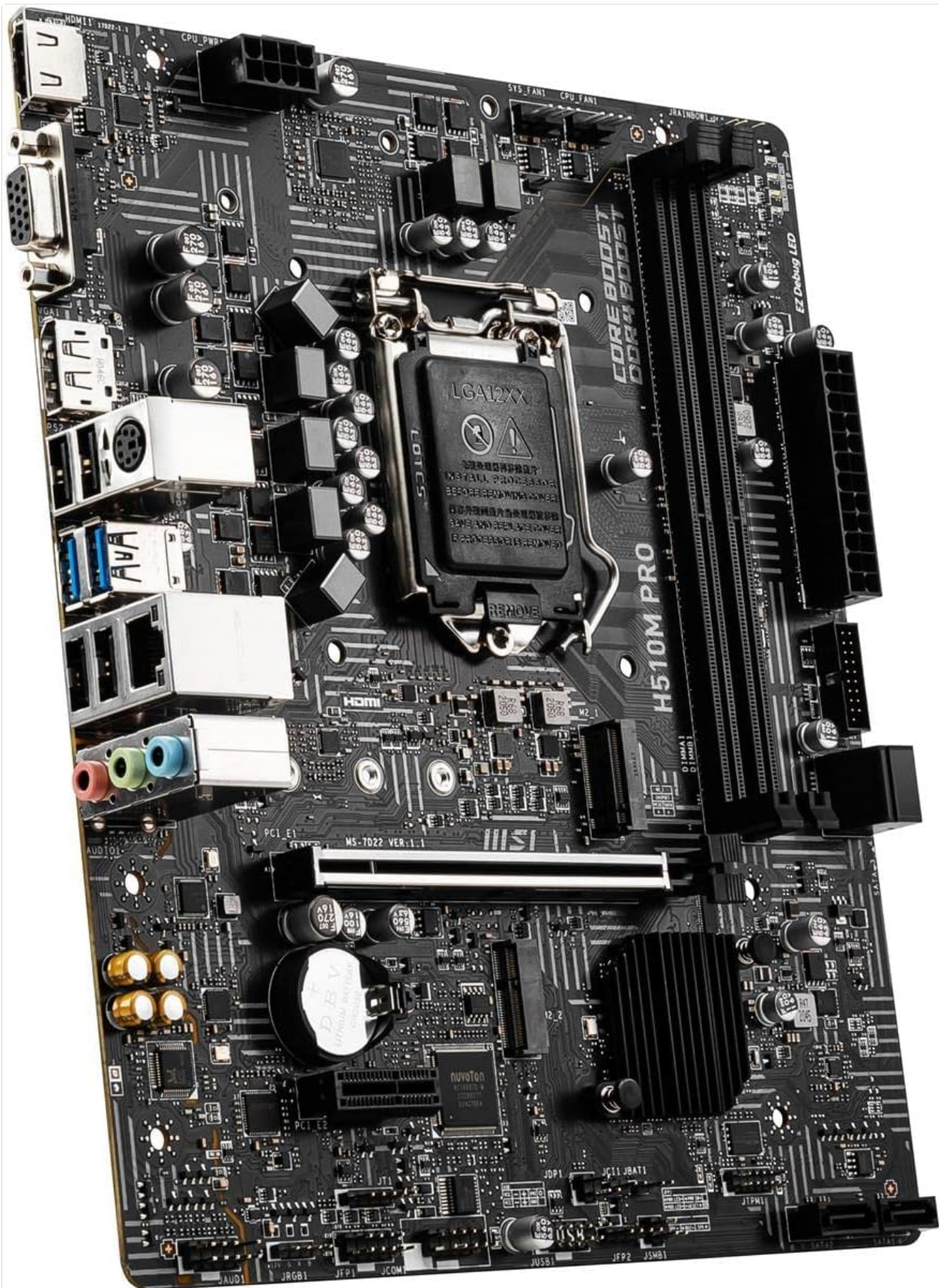
Figure 2.3: A top-down view of the MSI H510M PRO motherboard, showing the layout of the CPU socket, RAM slots, and PCIe slots.
