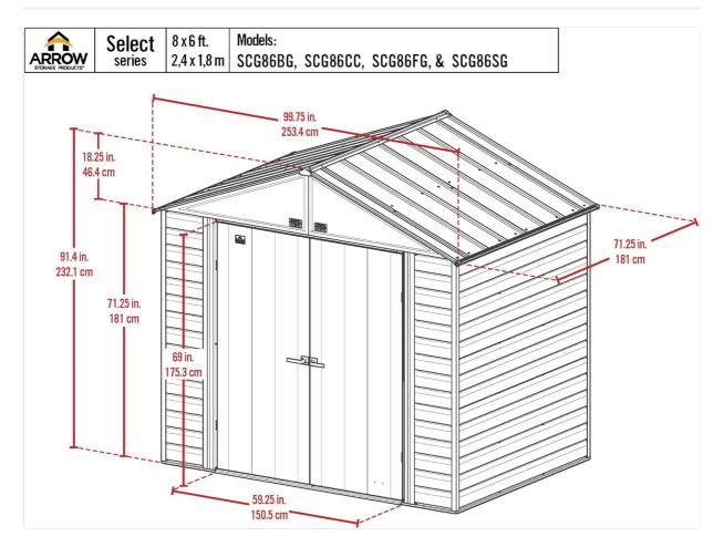
A detailed diagram illustrating the external dimensions of the Arrow Select 8' x 6' storage shed, including width (99.75 in / 253.4 cm), depth (71.25 in / 181 cm), height (91.4 in / 232.1 cm), door width (59.25 in / 150.5 cm), and door height (69 in / 175.3 cm).
