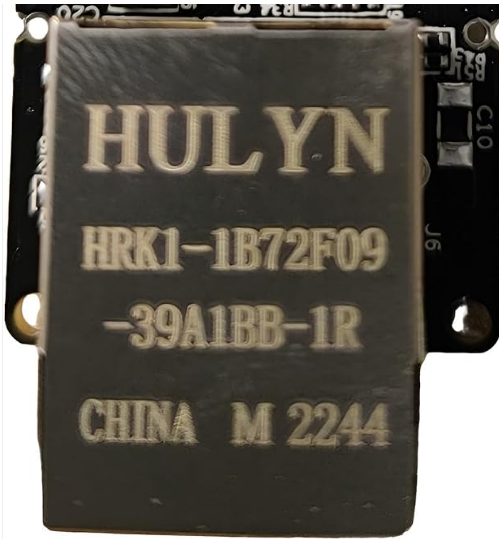
Figure 2.1: Detailed view of the WT32-ETH01 module, highlighting the integrated Ethernet port and main components.
