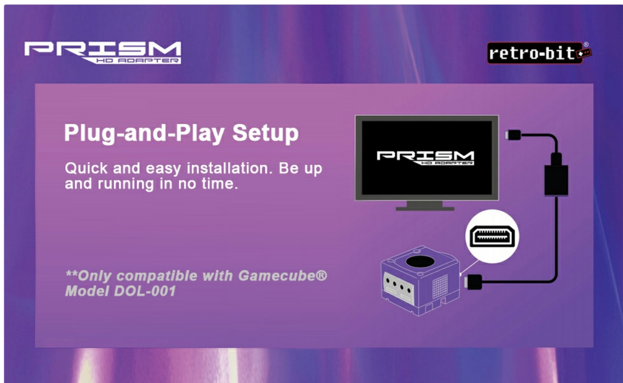
Image 3.1: Plug-and-Play Setup diagram. The adapter connects to the GameCube's digital AV port, and an HDMI cable connects the adapter to a display.
