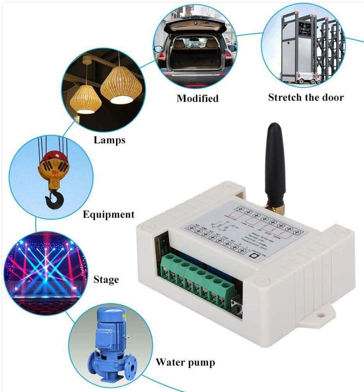
Image 1: Dpofirs 2CH 433MHz RF Remote Control Receiver Module with antenna and terminal blocks. This image shows the compact design of the receiver unit, highlighting its antenna and the screw terminals for wiring connections.
