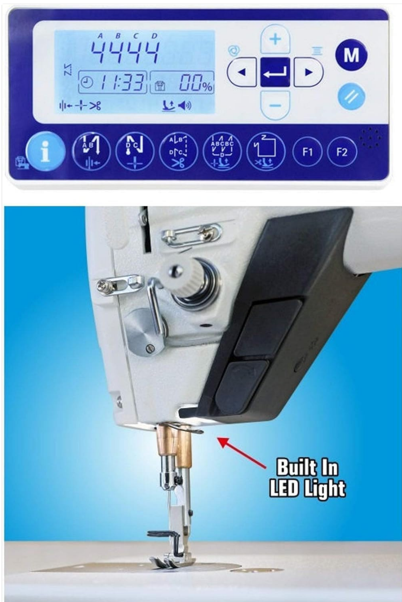
Image: Close-up of the JUKI DDL-8000A control panel and the built-in LED light illuminating the needle area.
