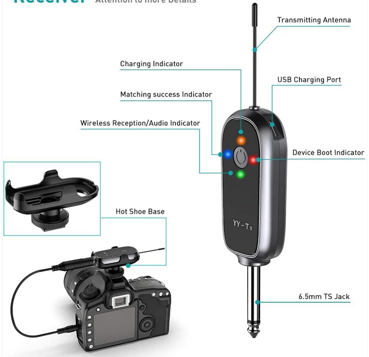
Image: Close-up of the receiver, showing its indicators, ports, and how it connects to a camera via the hot shoe base.
