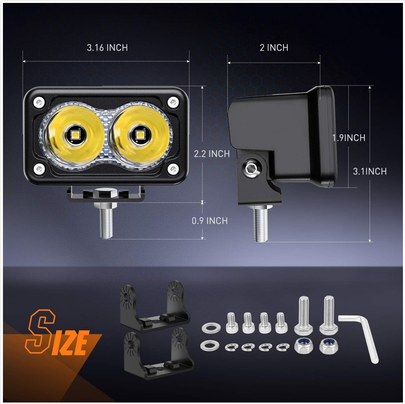
Image 3.1: Detailed view of the two LED light pods, their dimensions, and the included mounting brackets and hardware components.
