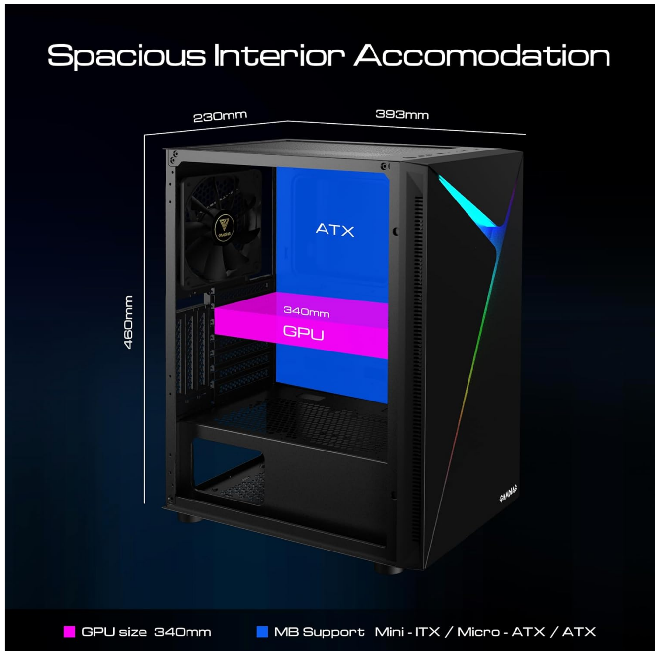
Figure 2: Interior dimensions and component support for the PC case.
