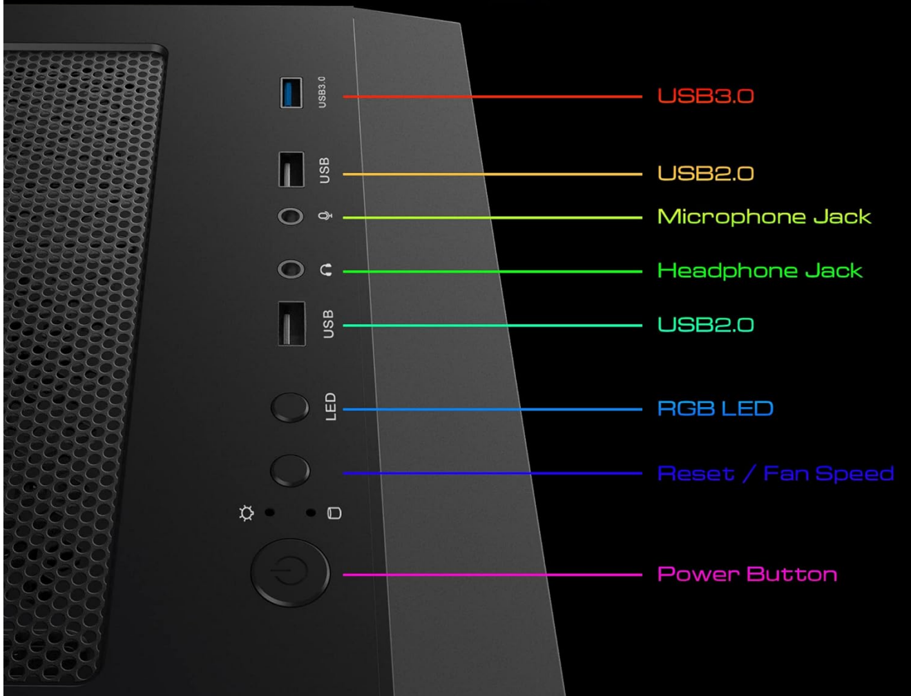
Figure 4: Front panel I/O ports and controls.
