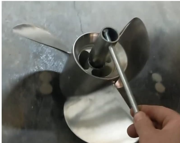
Image 3: The T-handle wrench being used to loosen the rear propeller nut for outer propeller removal.
