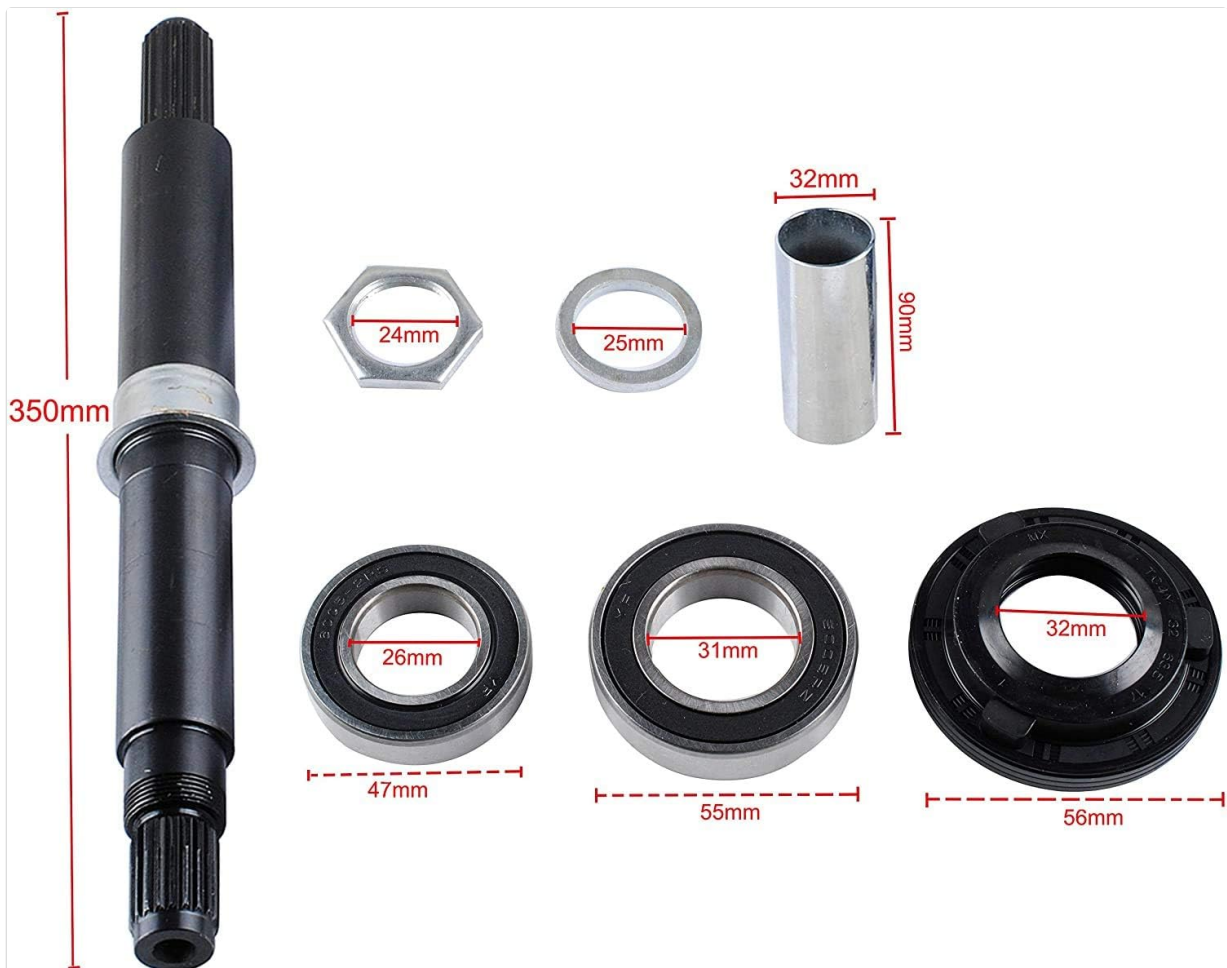
Image 2: Detailed dimensions of the Mintu Washer Bearing Kit components. This image provides measurements for the shaft (350mm length), nut (24mm), washer (25mm), sleeve (32mm diameter, 90mm length), bearings (26mm inner, 47mm outer; 31mm inner, 55mm outer), and seal (32mm inner, 56mm outer), aiding in component identification and compatibility verification.
