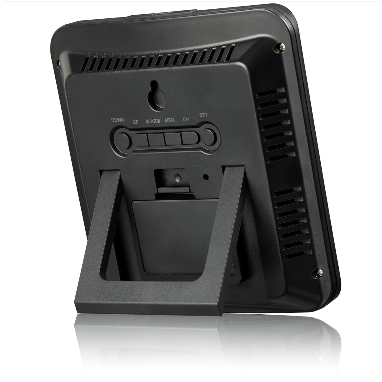
Figure 7: Rear view of the base station, illustrating the 'DOWN', 'UP', 'ALARM', 'MEM', 'CH', and 'SET' buttons, along with the integrated stand.
