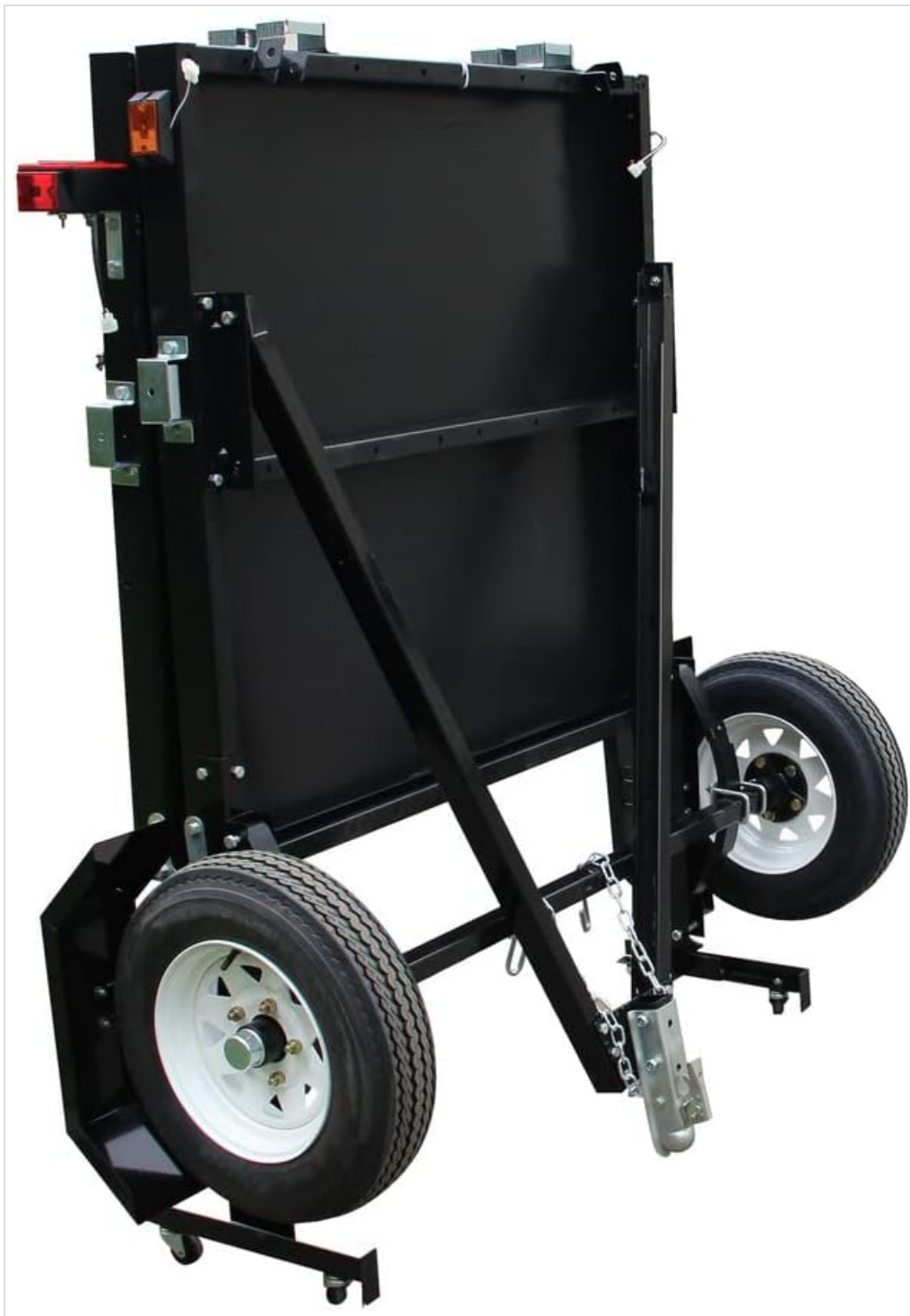
Figure 2: The trailer folded vertically, showcasing its compact storage capability.
