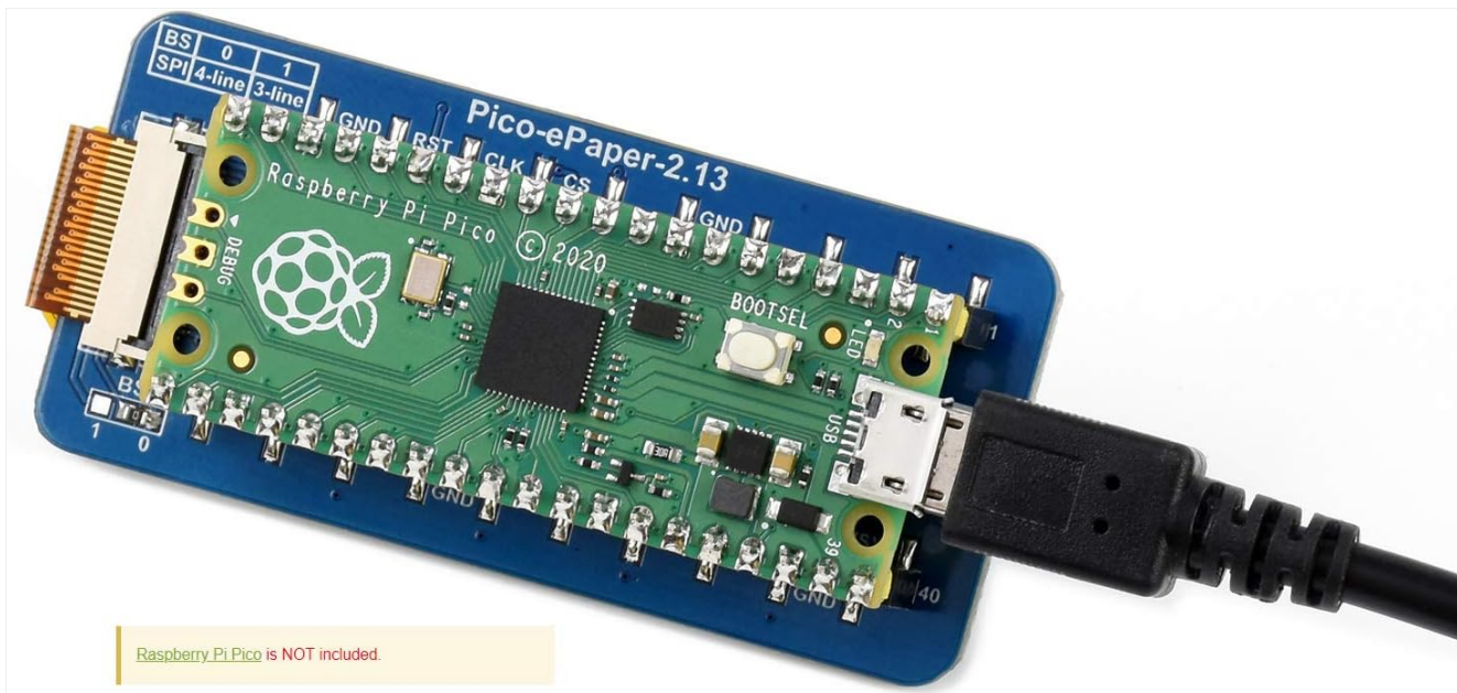
Figure 6: Raspberry Pi Pico with E-Paper module connected and powered via USB. Note: Raspberry Pi Pico is not included with the display module.
