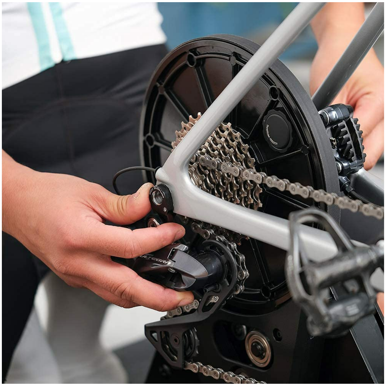
Image: Close-up of hands adjusting the quick release mechanism on a bicycle that is already mounted on the ThinkRider A1 trainer. This illustrates the final step of securing the bike.
