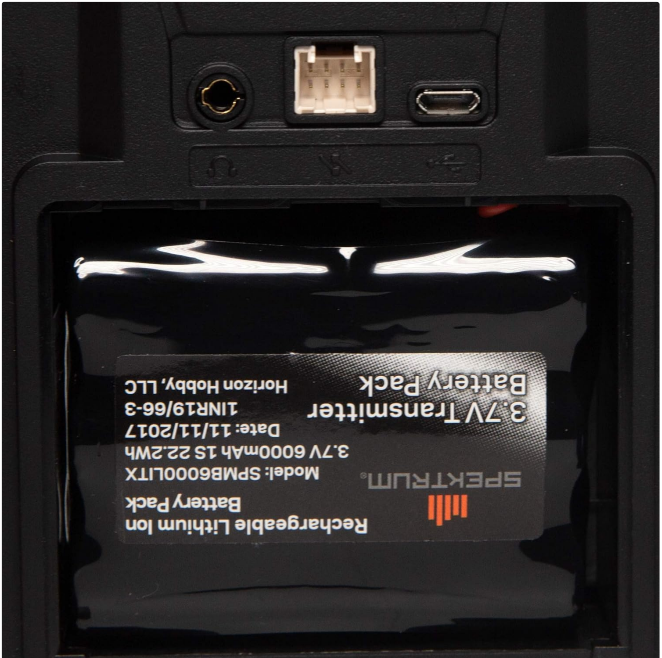
Figure 2: Rear view of the NX10 with the battery compartment open, showing the installed 6000mAh Lithium Ion battery.
