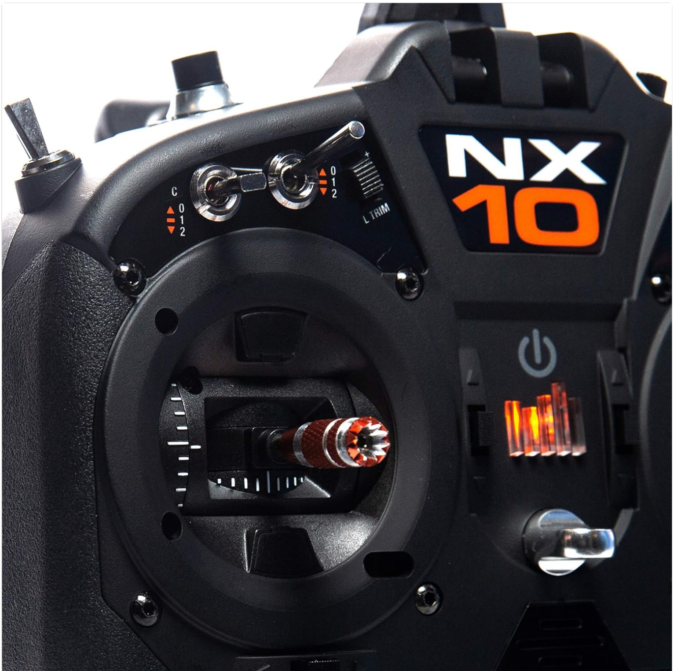
Figure 6: A close-up view of the Hall-Effect sensor gimbals, highlighting their robust construction and smooth operation.
