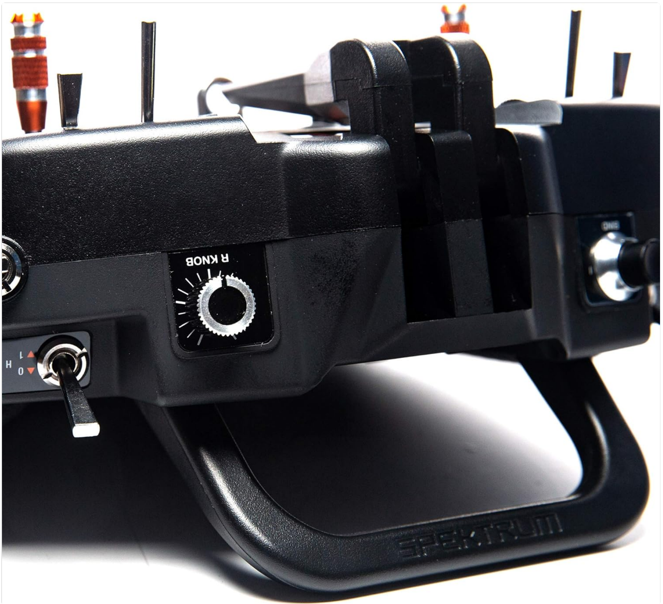
Figure 5: The bottom side of the NX10, illustrating the rotary knobs and sliders that can be assigned to different channels or functions.
