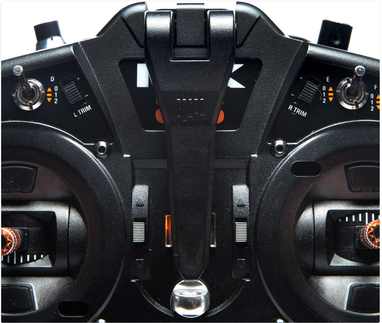
Figure 4: Top view of the NX10, showing the array of switches and trim levers for various functions.
