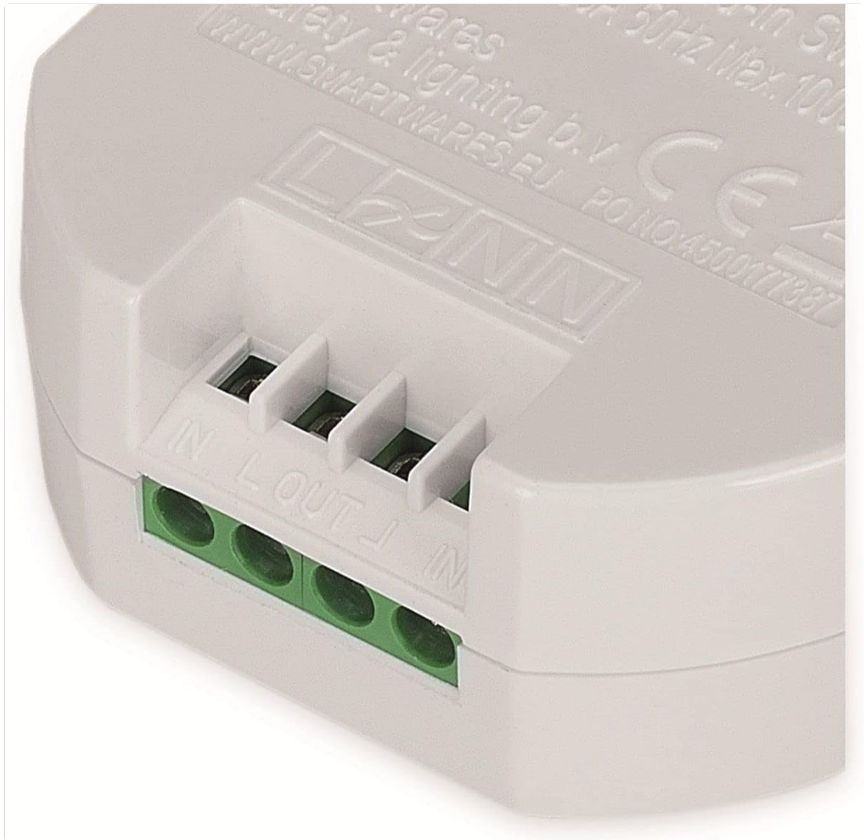
Image 4.1: Wiring terminals on the Smartwares receiver.
