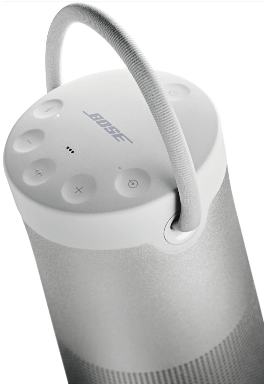
Figure 3: Speaker top controls for power, volume, Bluetooth, and multi-function.
