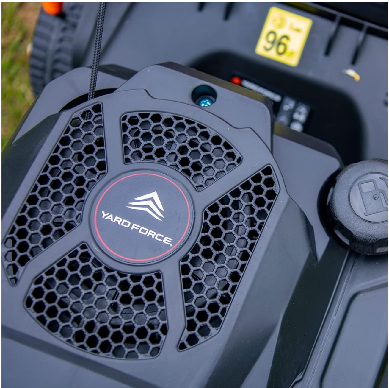
Figure 3: A detailed view of the mower's engine, highlighting the fuel cap and air filter cover, essential for pre-operation checks.
